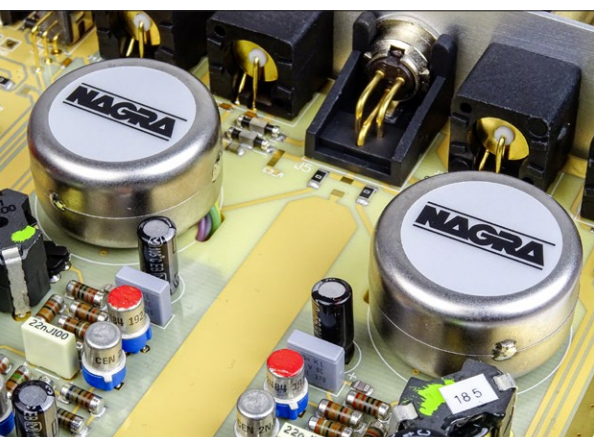
The encapsulated transformers are at the beginning of the signal path and are a Nagra specialty.
