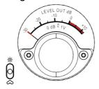
Nagra Modulometer is inherited from the second recorder developed by Nagra back in 1952, the Nagra II. The Modulometer is a typical Nagra precision instrument that displays the necessary information to perform the best possible recording. In the case of the CLASSIC PREAMP, the Modulometer displays the output level. The 0 dB corresponds to a 1 V rms signal on the output.
