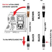
Start by removing the power cable from the C14 IEC Appliance inlet of the CLASSIC PREAMP. The Mains switch position is no longer relevant when an external power supply is connected.
