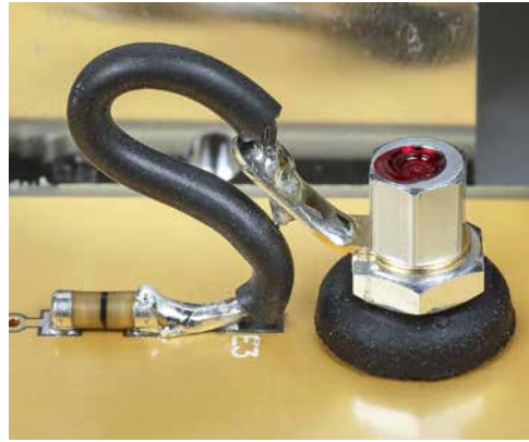
As is typical for Nagra, the circuit boards sit between small rubber dampers to protect them from microphonics. They call this „silence locked“.
