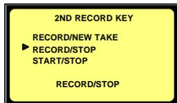
This sub-menu permits to select different modes for the red record side button. When selecting "**RECORD/NEW TAKE**", the action on the side button stays identical as for the keyboard record key. When selecting "**RECORD/STOP**", every time the red button is pressed once, the Ares-P/RCX220 toggles between record and stop mode.
