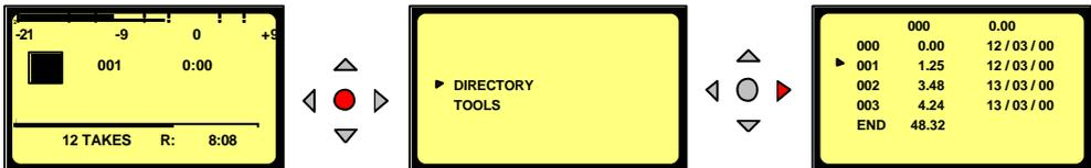
By using the “**UP**”, “**DOWN**”, “**LEFT**”, “**RIGHT ARROW**” keys ( 9, 11, 10, 12), once “**DIRECTORY**” has been selected, it becomes possible to scroll vertically and horizontally to view all the recorded files and their specifications.
