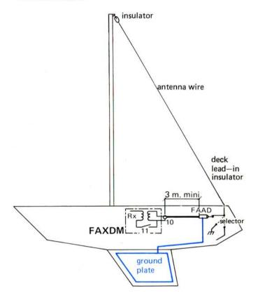
earth connection on the FAAD switch 11 on the FAXDM to "Off"
