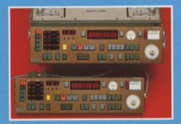
The keyboard is detachable and a second one may be connected to the machine, using an extension cable up to 50 m (150 ft) long.
