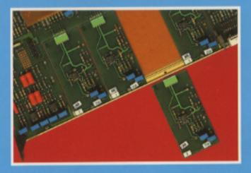
The section of the record amplifier that generates predistortion is implanted on a small plug-in circuit.
