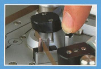
Once the splicing point is positioned on the playback head, the tape will be automatically advanced to the deckmounted scissors by the CUT function.
