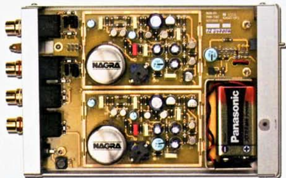
Inside the BPS—two transformers, one 9V battery.
