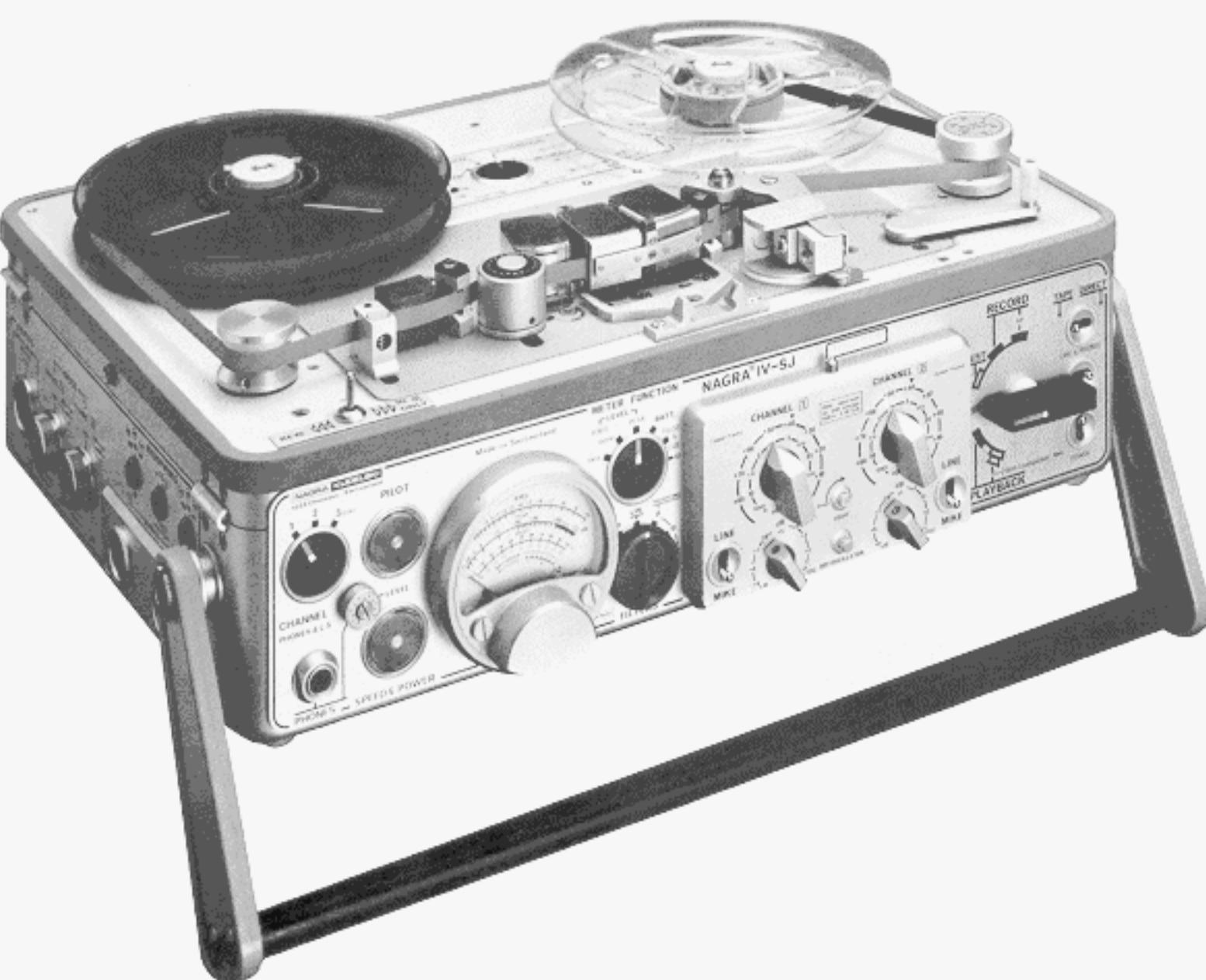
Four speed recorder: 15, 7½, 3¾ and 1½ in/s. Two direct recording tracks and one FM track. Application as a precision sound level meter when a measurement microphone is connected.
