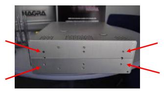
Step 1 Start by removing the transportation screws
