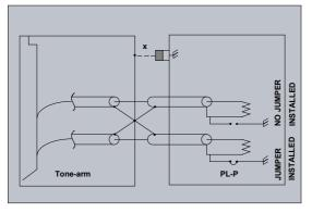
In this case be sure that only ONE of the two jumpers is installed. If you install both jumpers, you will immediately have hum again which will be louder or quieter depending on the distance left between the two cables linking the tone-arm with the PL-P. This is explained by the fact that doing this will form a loop which will pickup magnetic flux from adjacent equipment.
