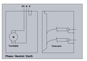
C. In the third case the tone-arm is mounted apart (as in B). However, the shielding wires from the cartridge are floating and are not connected together, or to the metal parts of the tone-arm.
