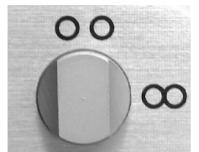
potentiometers are calibrated in logarithmic-scale and represent the amplification of the input amplifier, before the modulometer, for the corresponding channel.
