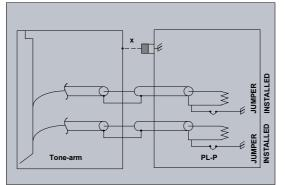
In this third case, both the jumpers are installed and the link between the two chassis "X" is obligatory.
