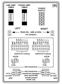
This diagram shows the different jumper positions for the various different options within the PL-P. To install a jumper, place it over BOTH of the pins of the corresponding selection so as to join them together.
