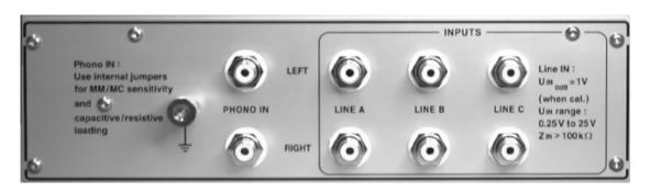
The left panel consists of four sets of stereo input connectors:
