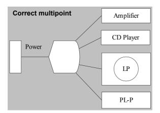
3. A third solution, which is equally viable, is to connect the individual units to the wall connector starting with the highest power consumers and finishing with the lowest power consumer and equally the units using high-level audio signals together and those with lower levels together, as indicated in the diagram below.
