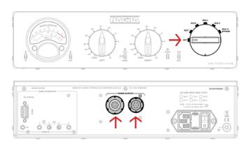
Repeat the procedure with the other ends of the umbilical cords, inserting them into the LEMO sockets at the back of the audio device chassis in the same way.
