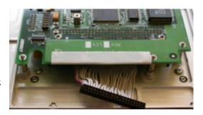
"A" twice 10 mm spacer & 1 shim, "B" one 5 mm spacer & 1 shim, "C" one screw & 1 shim.
