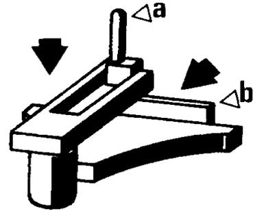
To rewind, turn the handle clockwise without pressing downwards so that the reels turn freely.
