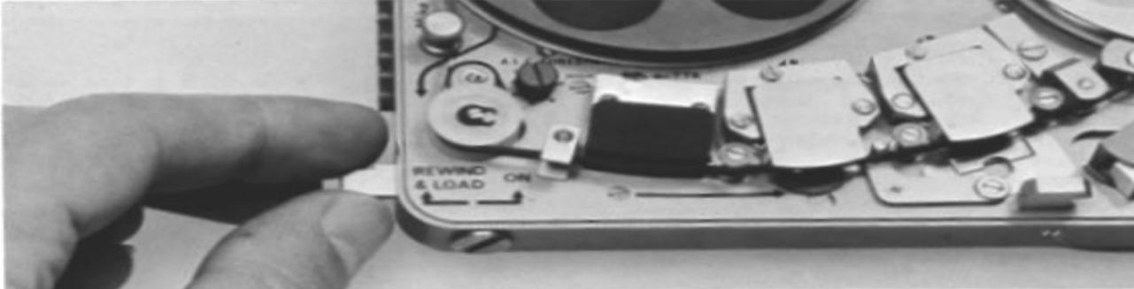
Ensure that reel fixations (6) are aligned with catches (Fig. 6) of the reel holders to allow the reels to be fitted easily.
