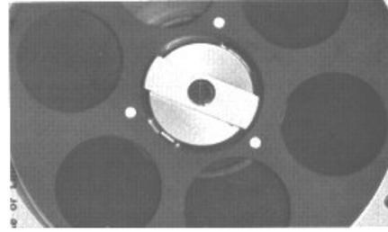
The tape is threaded as shown in Fig. 8, by passing the index finger through one of the holes closer to the centre of the reel, the tape is pressed against the reel holder. Then by slowly turning the supply reel clockwise, the tape is rewound until only a few millimetres extended beyond the point where it is held by the finger (Fig. 9).
