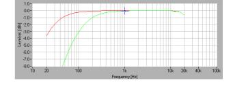
It is especially useful for recordings made using directional microphones outside in windy conditions, such as the green band stereo microphone. In fact, cardioid (speed capsules) such as the NAGRA microphones are susceptible to vortexes induced by wind moving round the microphone capsule, contrary to omni-directional (pressure) capsules, which are not.
