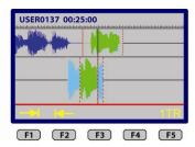
portion. In the above shown example, the right side of the green portion was too small. The closest marker was selected. In the second picture, the SHIFT key and the F2 key (left side) were pressed and hold and the jog wheel was turned to increase the length of this portion.
